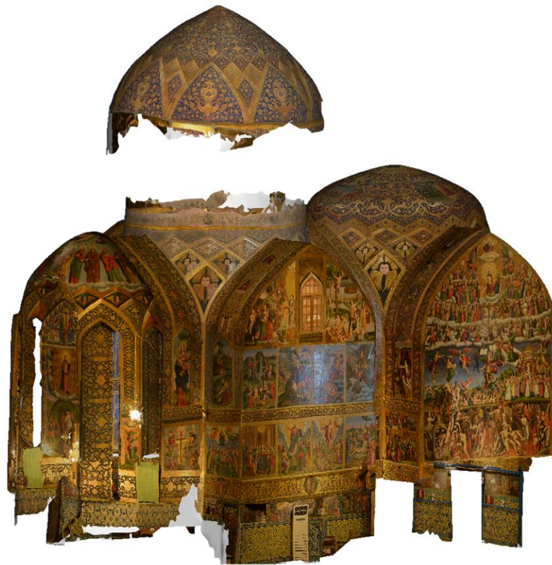
Figure 5. The entire meshed model with high-resolution textures representing frescoes; the lack of surface above the drum of the dome is obvious due to the impossibility to take pictures.
